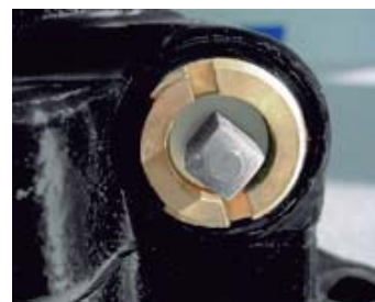
THE AUXILIARY VALVE IS OPERATED BY A SQUARE SPANNER
